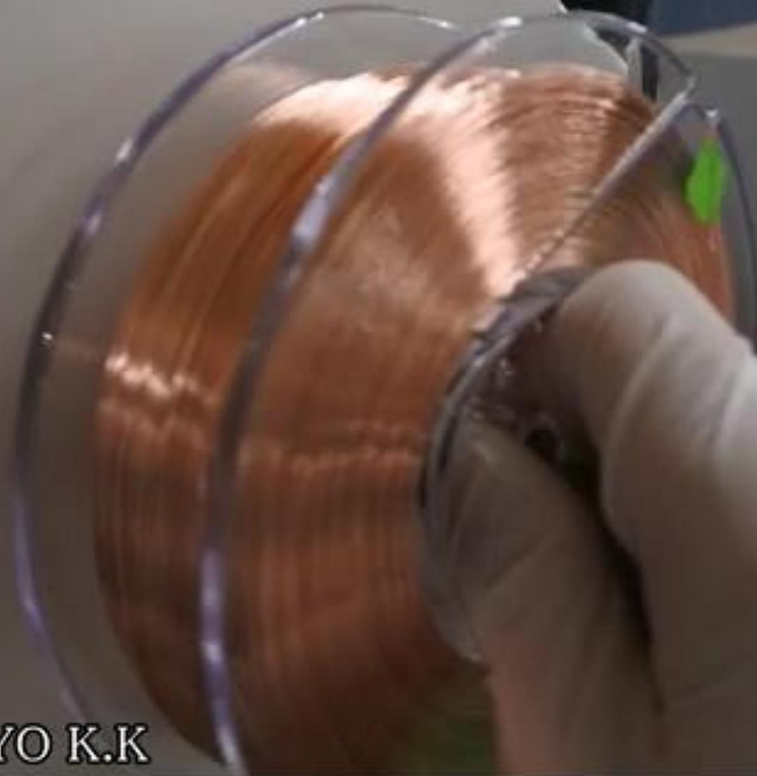
①Set the spool removed from the case to the bonding machine.
