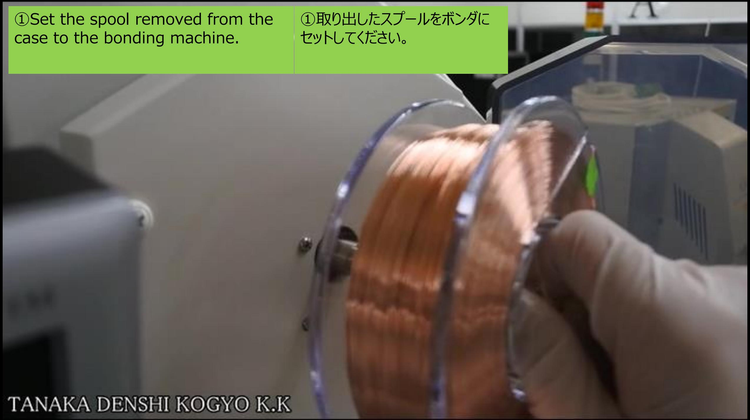
①Set the spool removed from the case to the bonding machine.
