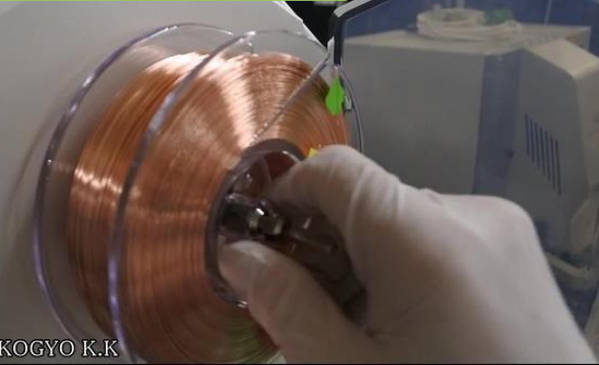
①Set the spool removed from the case to the bonding machine.
