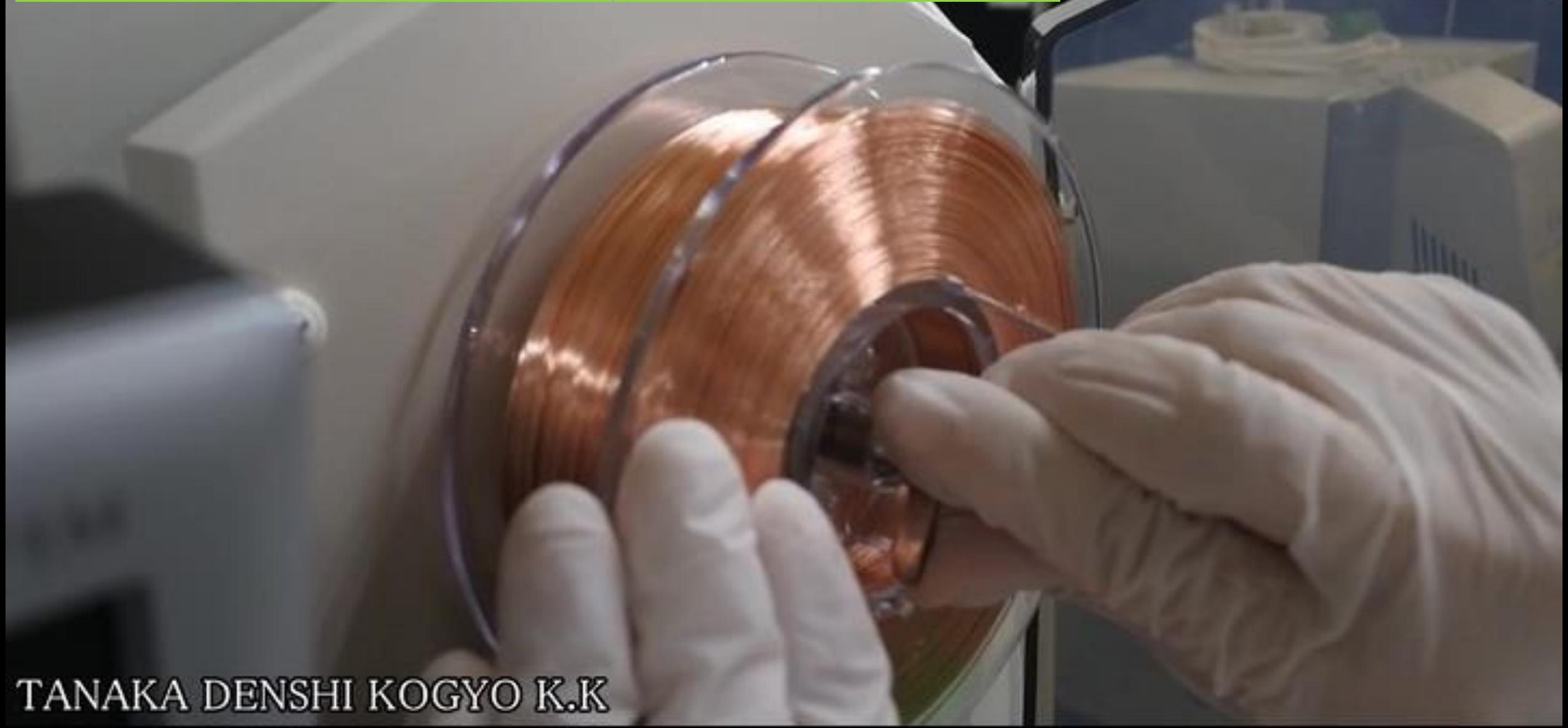
①Set the spool removed from the case to the bonding machine.
